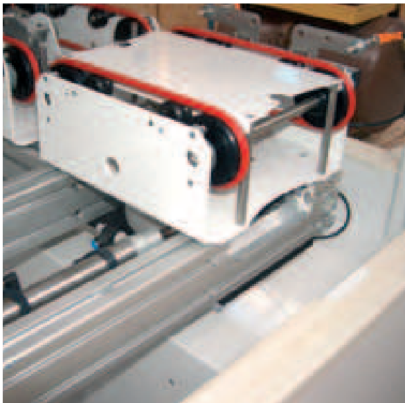
Handling and conveyance system for semiconductor transport/box.
