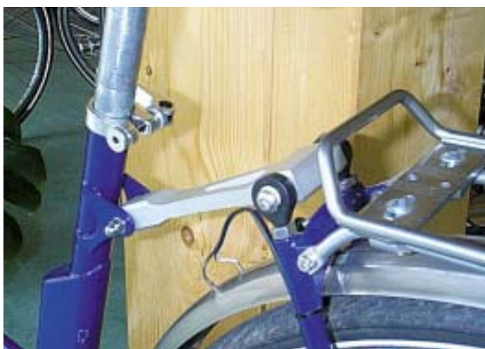
Picture 51.3: igubal® rod end bearings in the rear suspension mechanism of a bicycle
