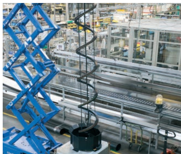
liftband test setup in the igus® in-house test lab
