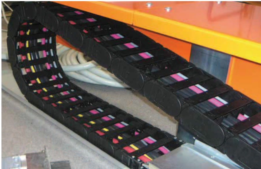
chainflex® CF2 cables are resistant to oil and coolants. e-chain®: System E4/00
