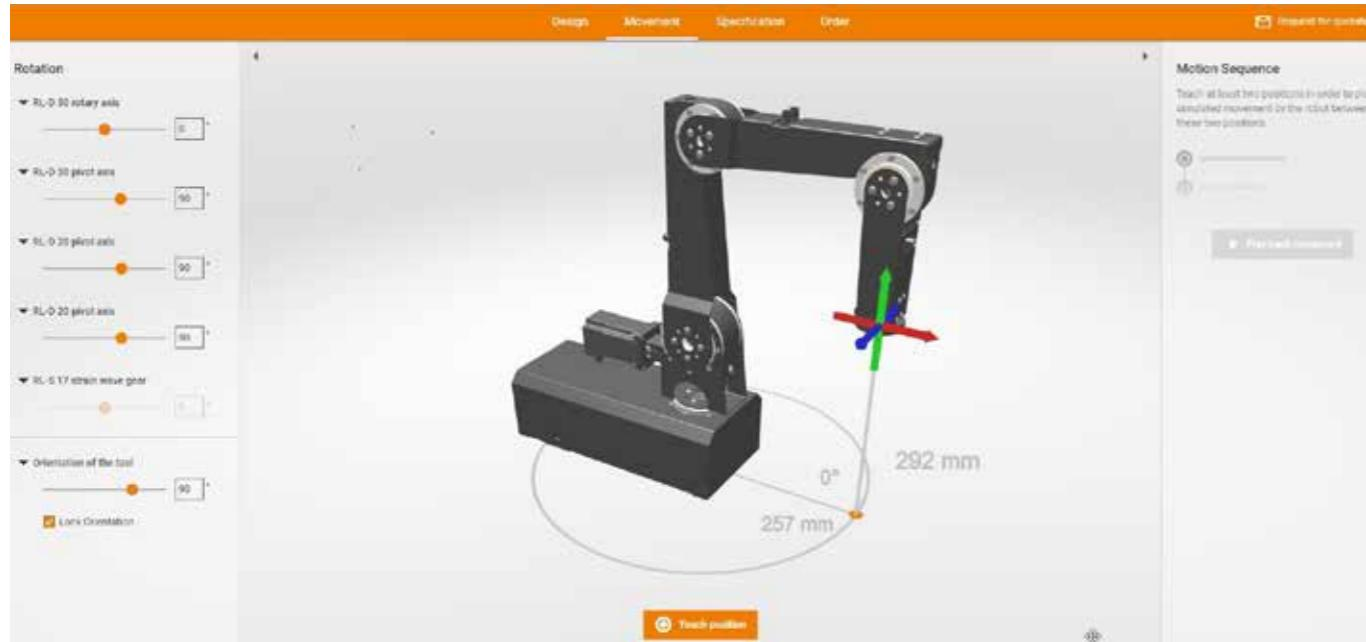
With the robolink® designer, you can quickly and easily configure online in an intuitive CAD interface your individual robolink® D robot arm online. Select individual robolink® components step by step to configure the robot arm individually, from the first axis to the tool. Simulation of the solution thanks to output of max. range and max. payload, teach function and inverse kinematics.
