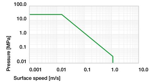
Diagram 01: Permissible pv values for iglidur® A180 plain bearings with a wall thickness of 1mm, dry operation against a steel shaft, at +20°C, mounted in a steel housing
