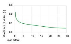
Diagram 05: Coefficient of friction as a function of the load, v = 0.01m/s
