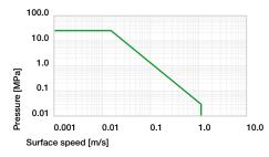
Diagram 01: Permissible pv values for iglidur® A180 plain bearings with a wall thickness of 1mm, dry operation against a steel shaft, at +20°C, mounted in a steel housing
