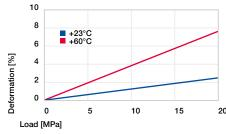
Diagram 03: Deformation under pressure and temperature
