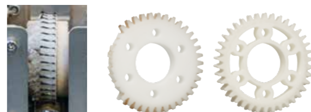
POM POM iglidur® I6 321,000 cycles 621,000 cycles 1 million cycles High wear Failed Low wear
