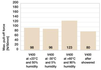
180° pull-off test after various exposure conditions
