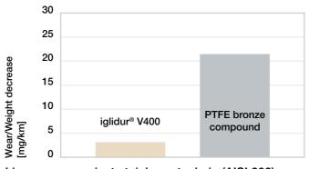
Linear wear against stainless steel pin (AISI 303) F = 35N, v = 0.5m/min
