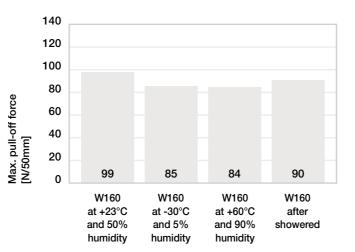
180° pull-off test after various exposure conditions
