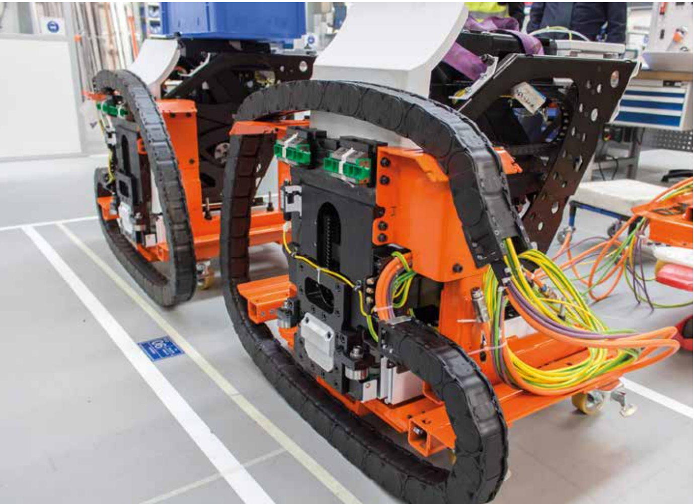
R4.1L e-tubes to guide motor, encoder and sensor cables on a bending machine
