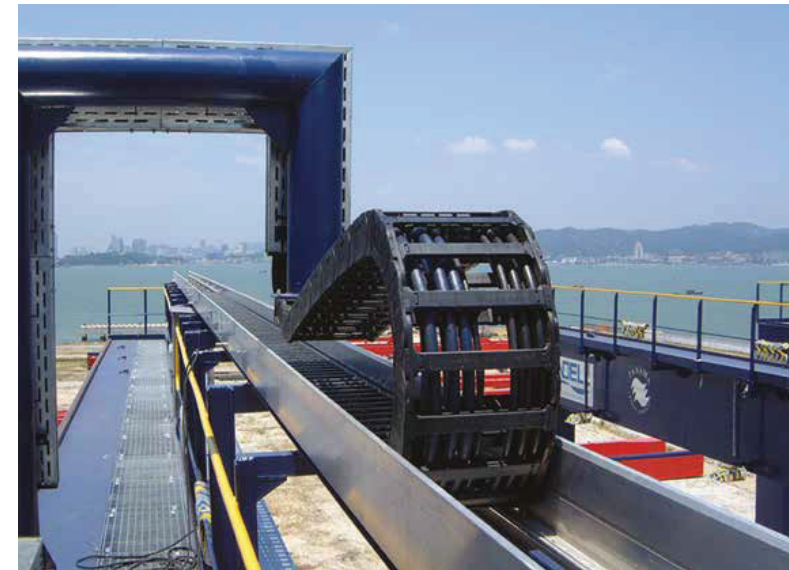
Series E4 in a seawater resistant igus® aluminium guide trough
