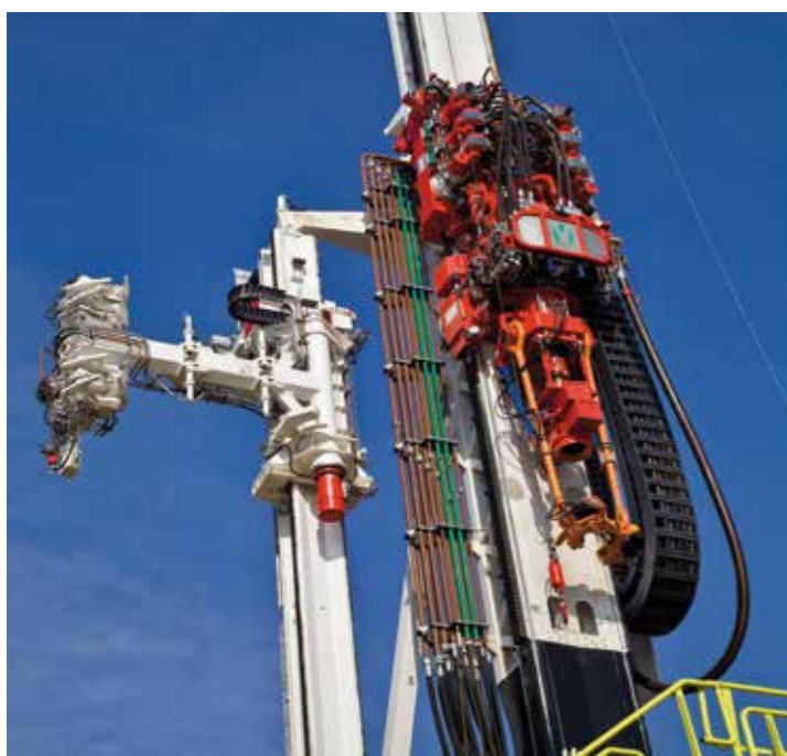
Compact design, custom configuration: two nested E4.112 e-chains® each around 12m long carry very heavy fill weights
