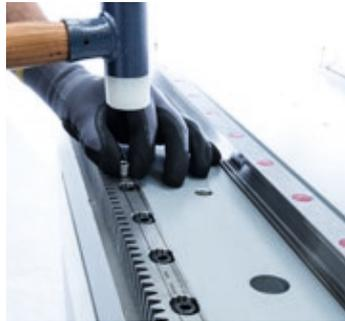
The assembly pin is driven into the pre-manufactured pin bore in the mounting base.
