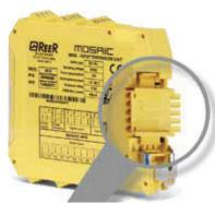
Mosaic MSC permits communication between the various units through a proprietary 5-way high speed safety bus. The MSC modular connectors can be used to connect the various expansion units to M1. The connectors are physically located on the back of each unit and are housed in the rail quide of the electrical cabinet.
