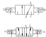
**Solenoid - Solenoid 5 ways 3 connections (Self-feeding)**
