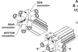
A = forward stroke connection B = backwards stroke connection M5 tube Ø4 and Ø6 fittings can be used for air connections. In case of use with 1600.16.01F mounting and REAR air connections use a 4mm pipe fitting.
