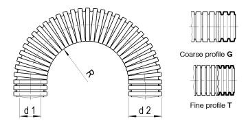
stat. R. = min. bending radius for static (fixed) installation
